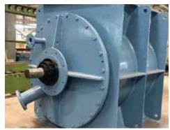
The body & rotor wears out due to heavy handling of material & it's abrasiveness. The gap between rotor blades & body increases making it difficult to control feed rate and smooth operation of rotor.
