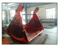
Manufacture and fabrication of ENDURAPLATES wear resistant plates by automatic, electronically controlled, open arc cladding process. Chutes, hoppers, liners, cyclones, ducts, casings etc. are some of the applications.
